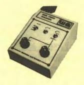
Using any source of composite video (colour or monochrome) and the Watford Beeb Video Digitiser, you can convert an image from your camera into a graphics screen on the BBC Micro.
